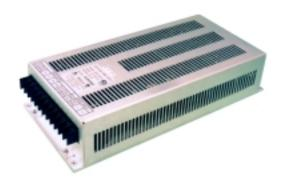
The BAP319 Series of DC/DC converters uses a field proven high frequency push-pull topology to generate 500W output power with convection cooling. Virtually any DC input/output combination is possible with short delivery times. The chassis-mount design features low component count and high efficiency. The use of high quality components and rigorous quality control results in an MTBF exceeding 200,000 hours at 45°C.
